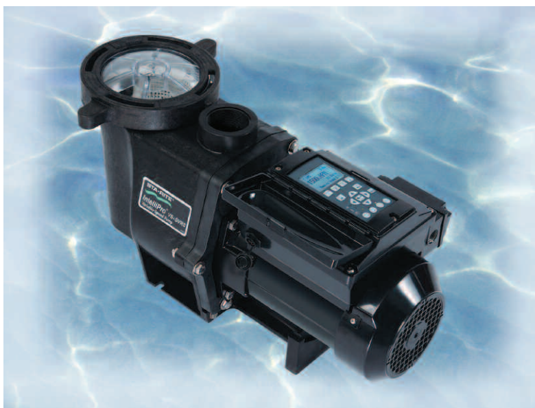
Multi-speed pool pumps like this one save energy by running at lower speeds for part of the day. Reducing the pump speed by half actually reduces the power requirement of the pump by three-quarters. Source: Pentair Water Pool and Spa, Inc.
